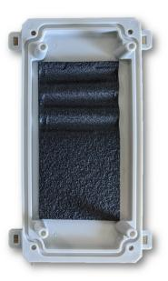
3. Once the batteries are replaced, gently remove the foam gasket from the lid of the monitor and place it in the grooves of the base.
